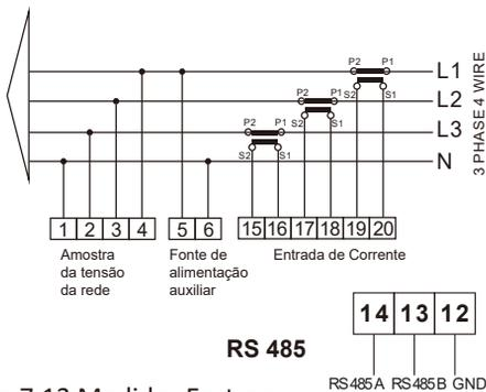
Eastron SDM630MCT Figura 7.13 Medidor Eastron
